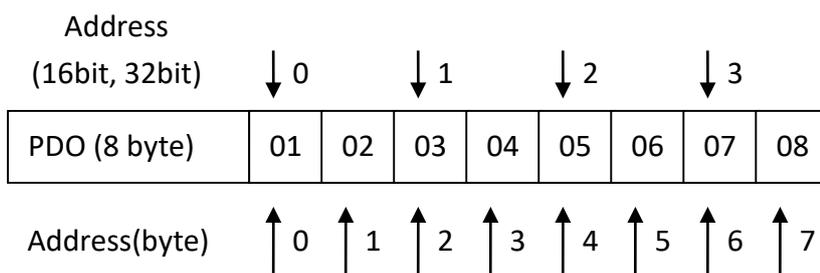
In accessing PDO data, one should select device types and addresses according to PDO data composition. Take TPDO\_1, which contains data as follows: 16bit, 8bit, 8bit, and 32bit, as an example as shown in the following figure.
