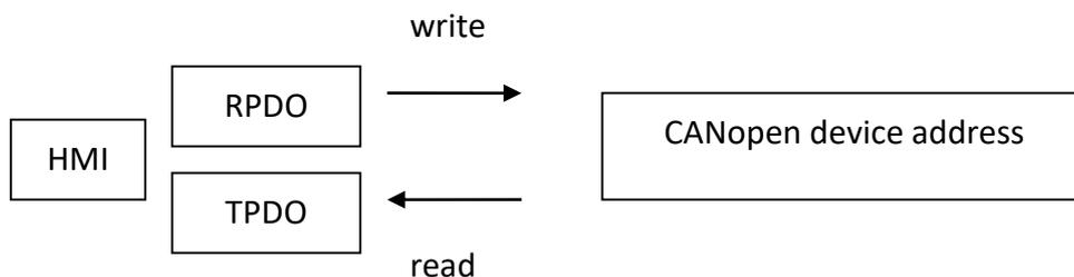
Use PDO to read or write CANopen device parameters.
