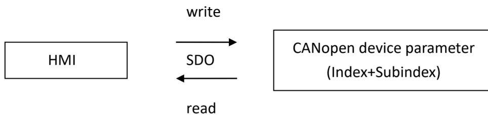
Use SDO to read or write CANopen device parameters.
