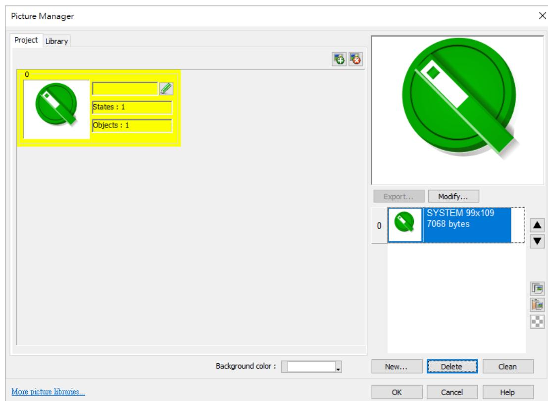
3. Then, repeat the process of copying the picture for state 2. This creates a picture for a two-position selector switch.
