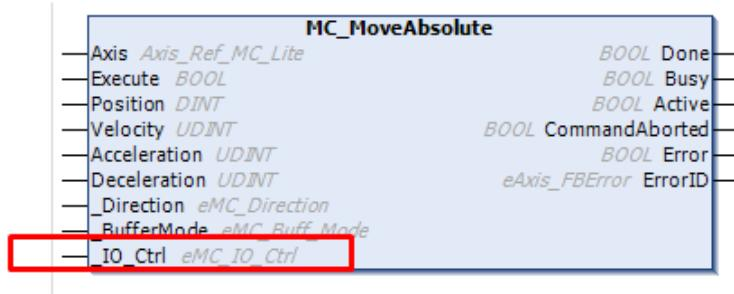
See settings of 558Fh and 559Fh in chapter 8. In 559Fh Motion Trigger Settings, three trigger signals can be pre-defined, and one of them can be used to trigger motion control when function block starts executing. In 558Fh Motion Output Settings, three output modes can be pre-defined, and one of them can be used after the movement is completed. "Done" can be configured either Blocking (digital output completed) or Non-Blocking(movement completed).
