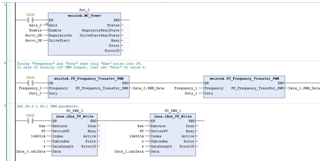
The result from Frequency\_Transfer\_PWM is written to the object – PWM Output Setting.
