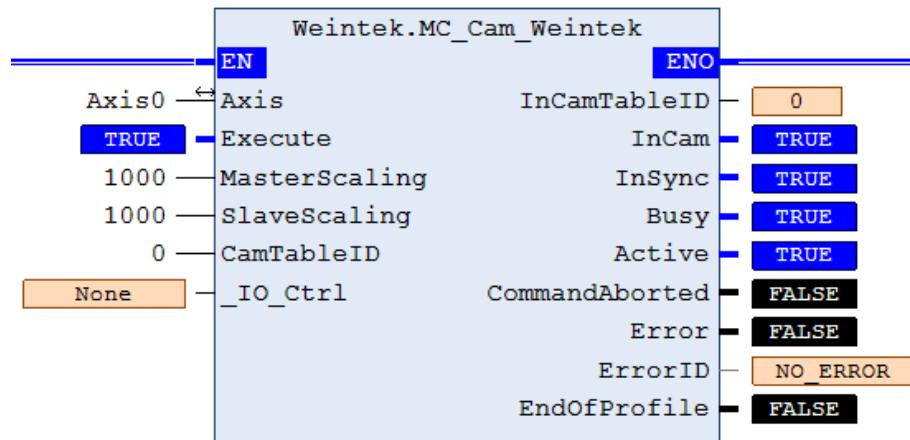
**MasterScaling:** The phase of the master axis is extended or contracted by using the specified scale. The unit is 1/1000.
