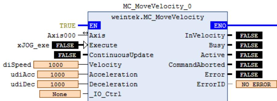
**Velocity:** Specify the target velocity and the rotation direction. Positive velocity = positive direction, negative velocity = negative direction.
