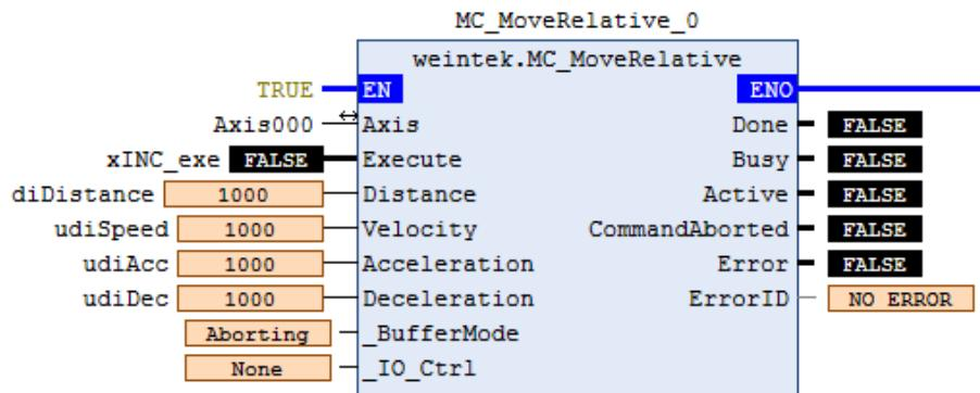
Distance: Specify the target position, which equals to current position + specified distance.
