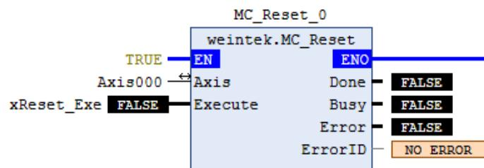
When an error occurs, MC\_Power.Error=TRUE, please execute MC\_Reset to change the axis state from Errorstop to Standstill, to continue operation.
