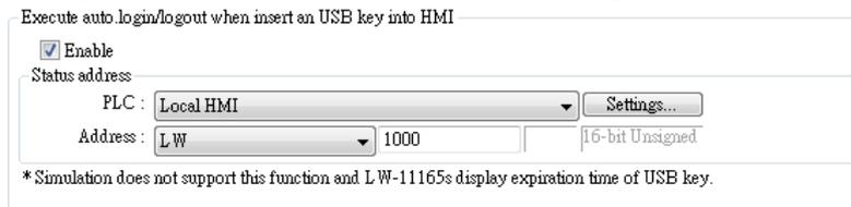
This function allows automatic login / logout using an USB security key. Insert the USB disk in which the key is saved to HMI to log in, and remove the USB disk to log out. The login / logout status will be written into a designated address, the result codes of login / logout:
