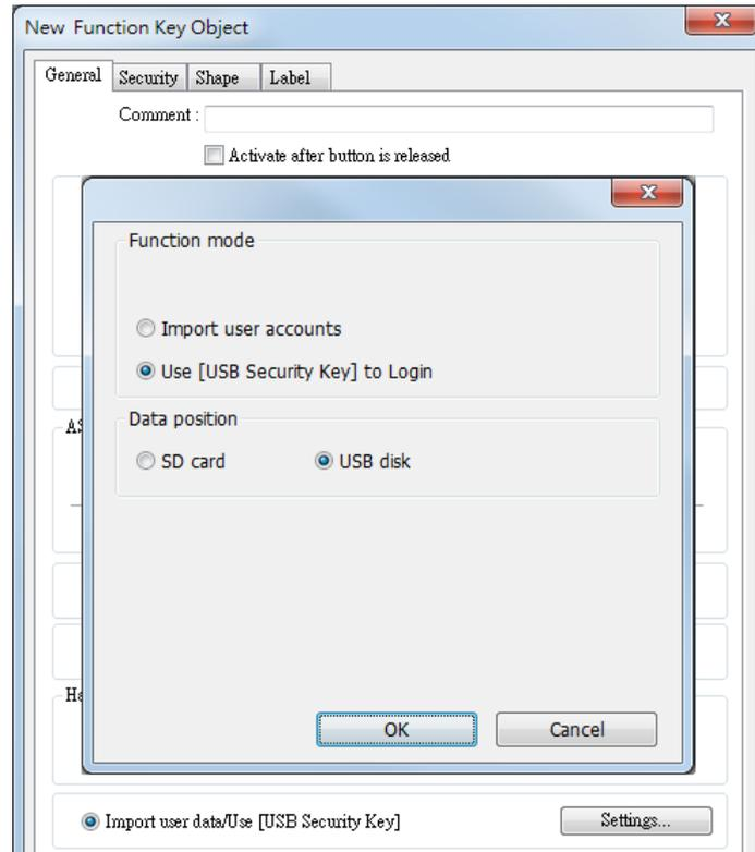
When finished, insert the external device to HMI, and press Function Key to log in using USB Security Key. If the [Effective Time] in Administrator Tools is specified, the login can only be done in the time limit specified. The system will log out automatically when the key expires.
