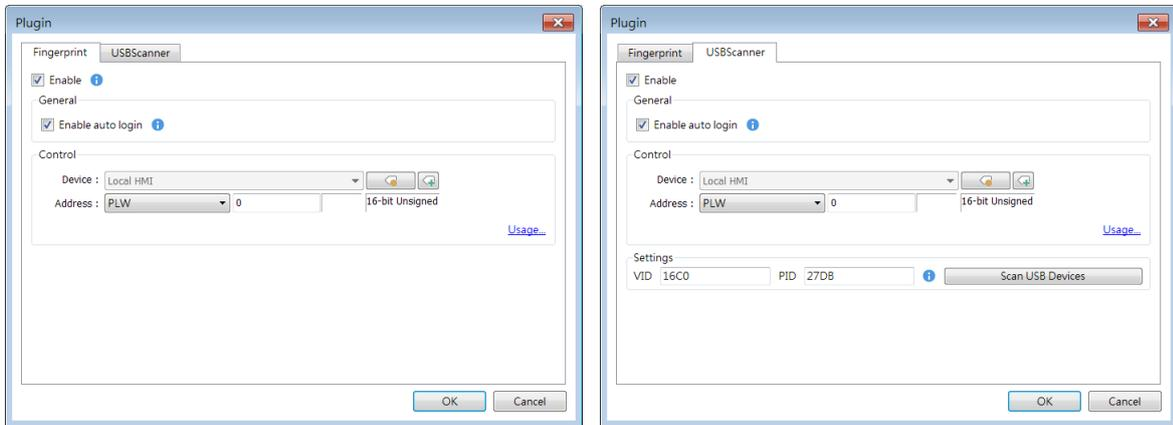
When configuring the USB scanner, to prevent interference from other USB devices during login, it's necessary to first set the VID and PID of the USB scanner. After clicking [Scan USB Devices], the system will prompt a message "Please insert your USB Device". Once the USB scanner is inserted into the PC, the system will obtain a unique VID and PID for the USB scanner. Click [Save], and the system will automatically incorporate this VID and PID into the settings.
