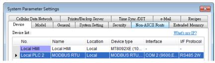
In the setting page of each object, select "MODBUS RTU" in [PLC name], and set the address of MODBUS RTU.
