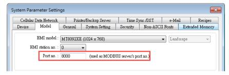
3. When finished, MODBUS Server is listed in [Device] tab. The configuration of MODBUS device is completed. Compile the .emtp file and download the compiled .exob file to the HMI, then HMI data can be read or written by using MODBUS protocol.
