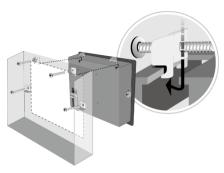
Minimum required clearances (along the overlay): Top / Bottom / Sides 15 mm Maximum panel thickness: 4 mm
