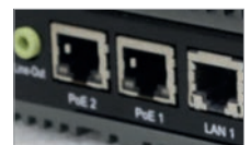
2 x PoE ports with Intel GT210AT Controller
