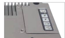
OSD on the rear side
