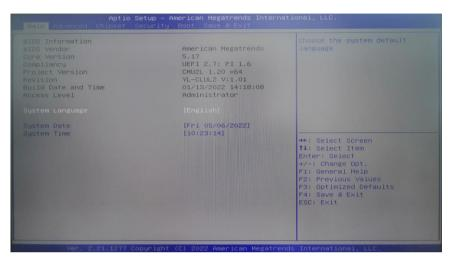
After the device starts, press the "Delete" button to enter the BOIS setting interface.
