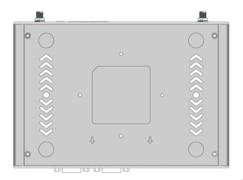
After finish installing the internal parts, then install the bottom plate and install the M2.5\*6 screws.
