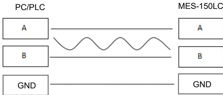
RS485 transmission distance does not exceed 600 meters.
