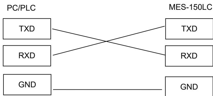
RS232 transmission distance does not exceed 15 meters
